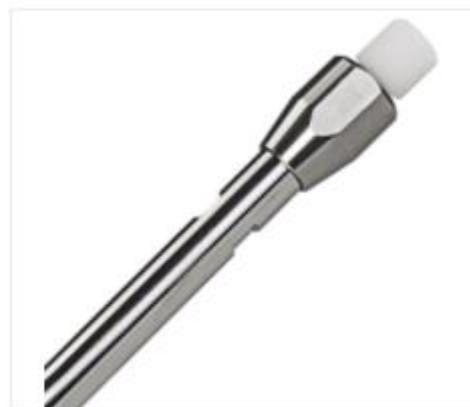
Colonne HPLC EC (analytique), NUCLEOSIL 120-3 C18, 3 µm, 125x4.6 mm
