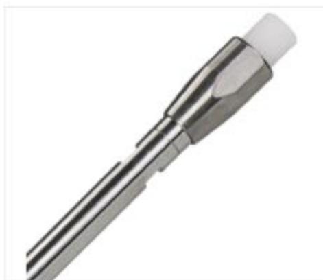
Colonne HPLC EC (analytique), NUCLEODUR C18 Gravity, 5 µm, 250x4.6 mm
