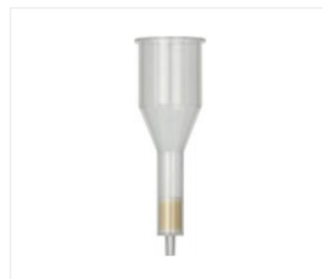
Colonnes SPE LV, CHROMABOND HR-X, 85 µm, 15 mL/200 mg
