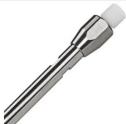
Colonne HPLC EC (analytique), NUCLEOSIL 100-5 NH2, 5  $\mu\text{m}$ , 250x4.6 mm
