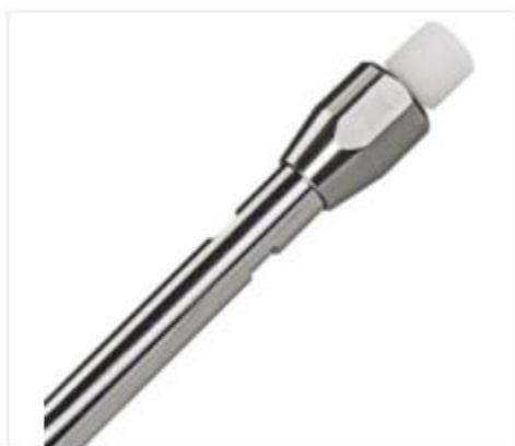
Colonne HPLC EC (analytique), NUCLEOSIL 100-7 C18, 7 µm, 150x4.6 mm
