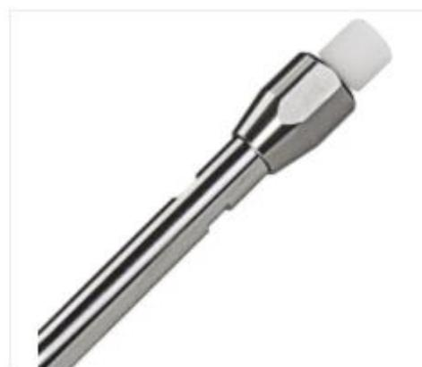
Colonne HPLC EC (analytique), NUCLEOSIL 120-3 C18, 3 µm, 100x4 mm
