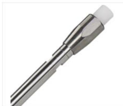
Colonne HPLC EC (analytique), NUCLEODUR 100-5 C18 ec, 5 µm, 150x4.6 mm
