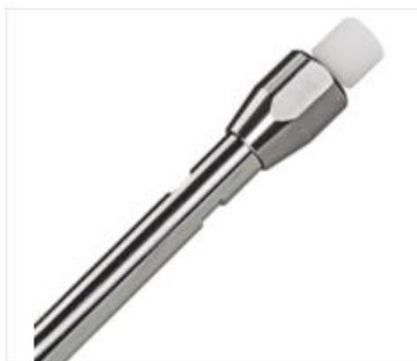
Colonne HPLC EC (analytique), NUCLEOSIL 100-5 C18, 5 µm, 150x4 mm
