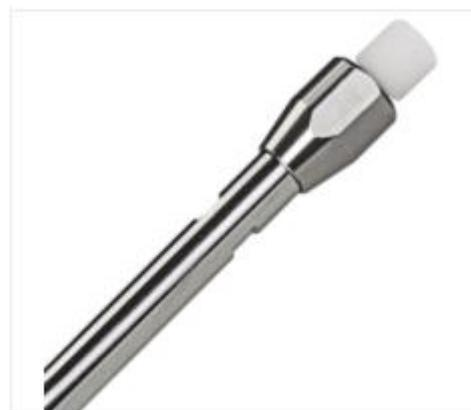
Colonne HPLC EC (analytique), NUCLEOSIL 120-5 C18, 5 µm, 250x4 mm
