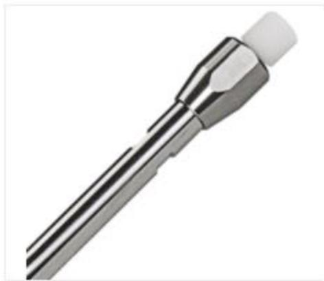
Colonne HPLC EC (analytique), NUCLEOSIL 120-5 C18, 5 µm, 125x4 mm
