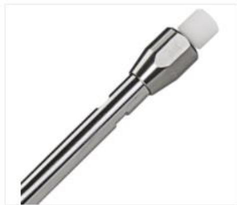
Colonne HPLC EC (analytique), NUCLEOSIL 100-5 C18, 5 µm, 125x4 mm
